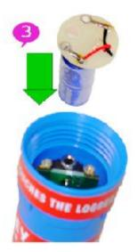
4. Screw the two socket head screws into the sockets on the logger board. Make sure that the star shake-proof washers are on the socket head screws. When the socket head screws are replaced they should only be tightened until they are firm. Over tightening may damage the logger.
