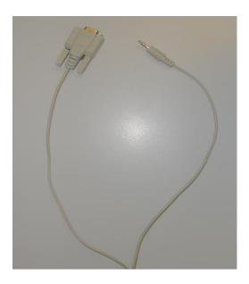
Connect the female DB 9-pin female connector of the serial interface cable to the 9-pin male serial port (COM port) on the computer and plug the stereo plug into the stereo plug socket of the data logger as shown in the picture.
