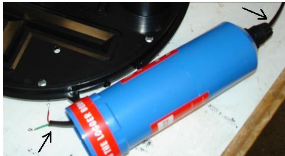
3. Using a small screwdriver, attach the wires to the screw terminal connector on the PCB as shown below.
