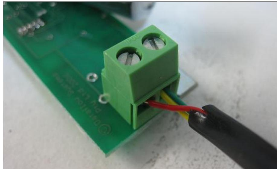
4. Carefully push the PCB back into the housing whilst gently pulling the cable through the other end. Tighten the cable gland.
