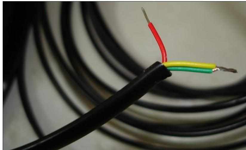
2. Separate the wires into two pair's red/black and green/yellow. The black wire is not essential and can be cut off completely.
