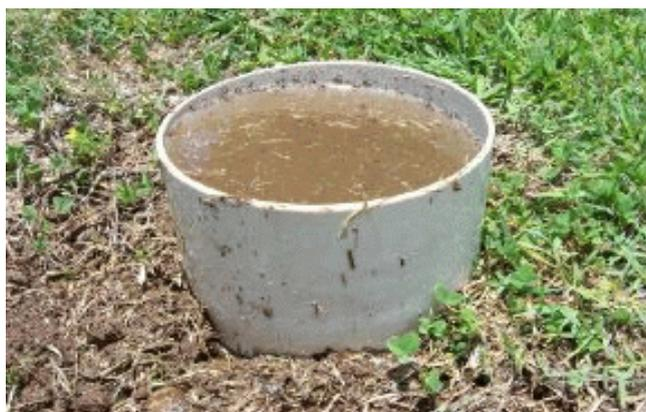
One simple way to achieve this is to either, place a piece of PVC pipe on the point where the access tube is going to be installed or form a soil dam around the site. Then fill the soil dam or container with water. The water must be allowed to drain away before you refill the container. The dam or PVC pipe must be filled a number of times to ensure that the soil is wet all the way down to the depth that the access tube is to be installed.
