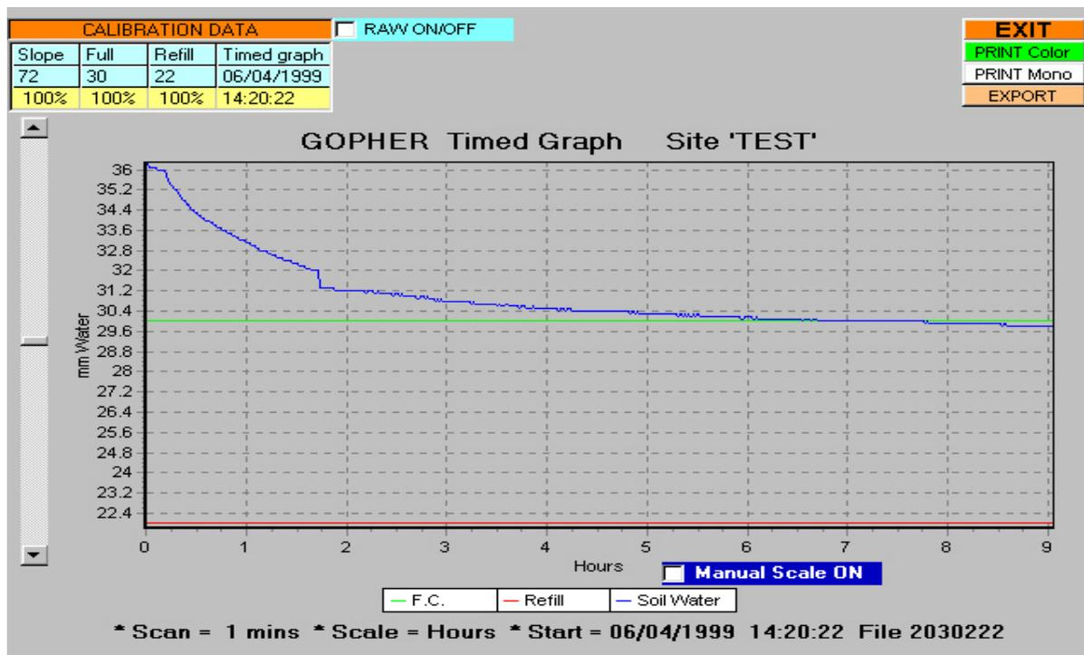
Timed recording can be used to provide detailed recording of water use against time. The graph illustrated was used to measure the field capacity of the soil when drainage had ceased. Water use, recharge rates and wetting fronts can be measured and viewed with this graphing mode.
