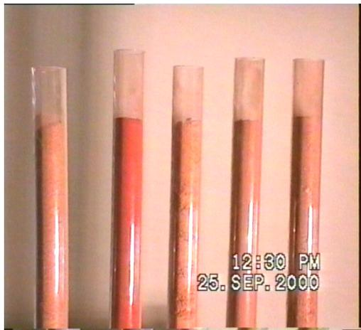
This picture shows five (5) different soil types being tested. The container for the soil is 25mm Acrylic tube. This tube can be purchased from Soil Moisture Technology.
