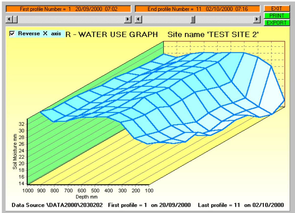
This is a three dimensional representation of all profiles for a site, a pictorial view of the soil moisture movement in the soil.
