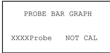
The horizontal bar graph displays graphically the moisture levels read by the probe.
