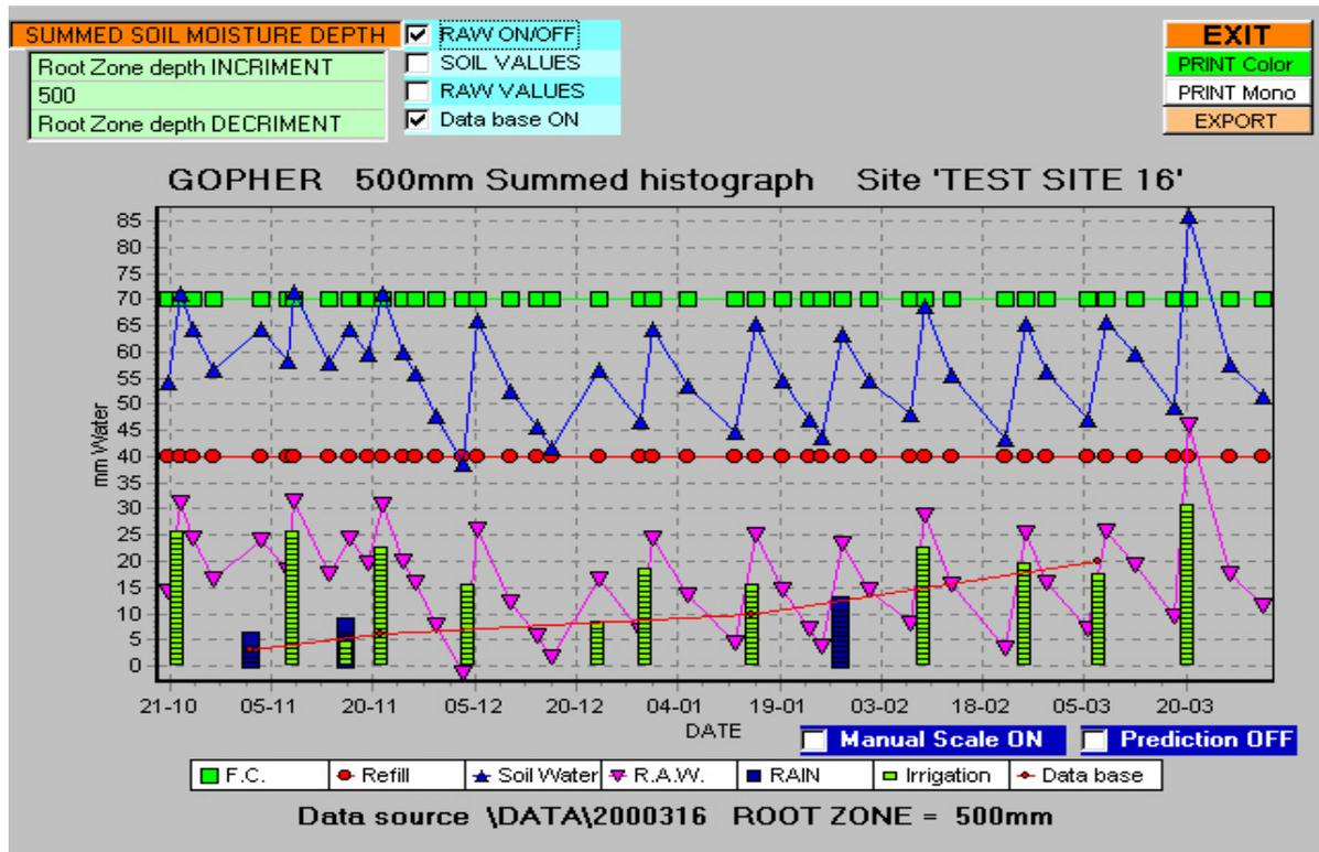
This graph displays the sum of the profile points down to the nominated root zone for all the profiles for a selected site. The depth of the summed soil moisture can be changed by clicking on the 'Root Zone depth INCREMENT' or Root Zone depth DECREMENT'.
