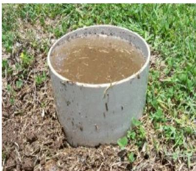
If the access tube installation is a new site then the easiest way to install the access tube is to saturate the soil before installation. This is very important in clay soils. Dry clay can be very hard and also sticky. This will make the access tube installation very difficult. However if the clay soil has been saturated then the installation of the access tube will be easy because clay when it is wet is very slippery.
