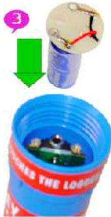
4. Screw the two screws into the sockets on the logger board. Make sure the shake-proof washers are re-installed. When the screws are replaced they should only be tightened until they are firm. Over tightening may damage the logger. If the logger is fitted with a status LED, this will flash 4 times to indicate the logger has been re-powered.
