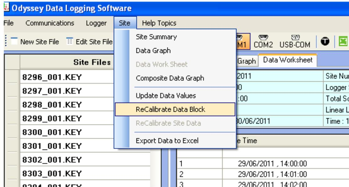
4. If you are downloading a new data block the calibration settings will automatically be applied to your data without the need to recalibrate the data manually as per steps 1 to 3.
