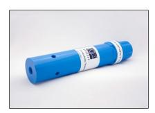
The Odyssey Conductivity and Temperature recorder encapsulates both the logger and sensors in one water proof housing. The conductivity of the water is measured by induction that alters the signal coupling between two sensor elements. At the same time temperature measurements are taken in order to calculate and output the conductivity measurements temperature corrected to 25°C.
