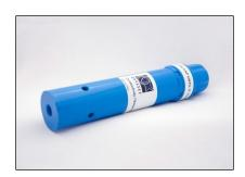
The Odyssey Conductivity and Temperature recorder encapsulates both the logger and sensors in one water proof housing. The conductivity of the water is measured by induction that alters the signal coupling between two sensor elements. At the same time temperature measurements are taken in order to calculate and output the conductivity measurements temperature corrected to 25°C.
